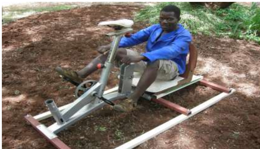
Figure 1. Bicycle component of a human-power shredder [10].
