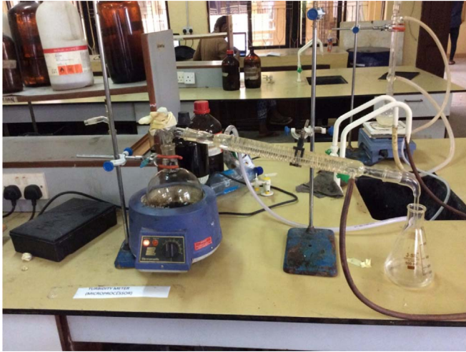
Fig. 1. Atmospheric distillation of oil for dehydration.
