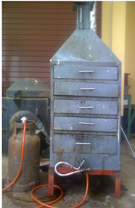
Fig. 2. Pictorial view of the gas-fired cabinet dryer.
